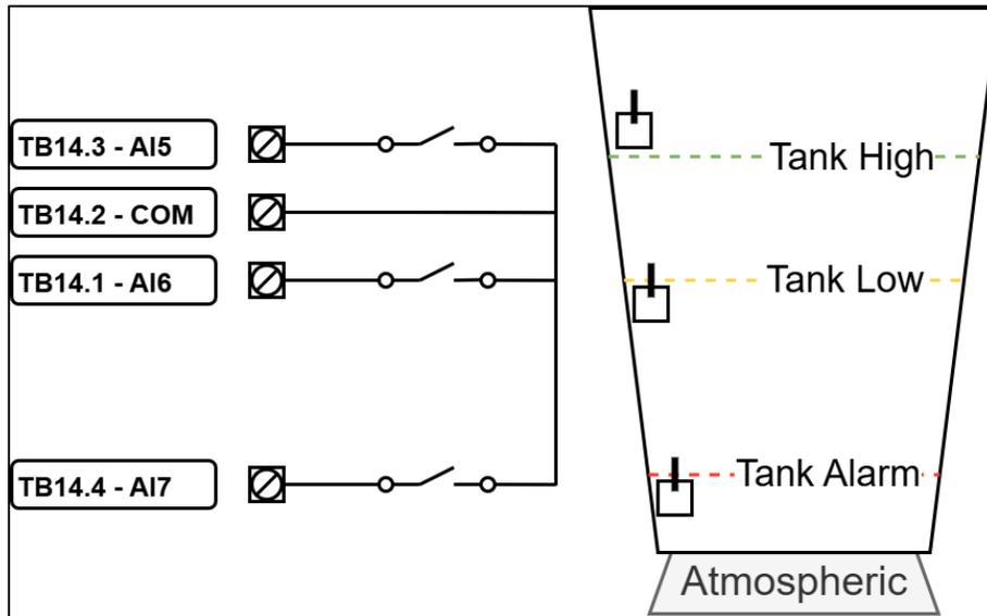
Illustration 13 - Atmospheric Tank Float Level
