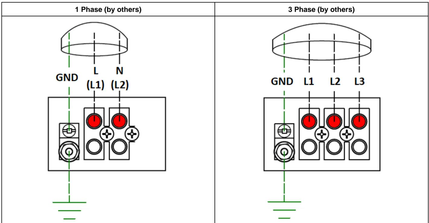
Illustration 14 - One and Three Phase Power Supply Connections
